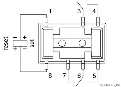
Contacts are shown in reset condition. Contact position might change during transportation and must be reset before soldering.
