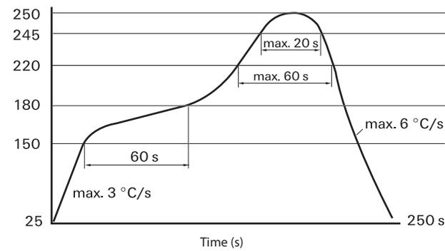
Resistance to soldering heat - Reflow profile
