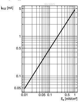
Photocurrent <sup>4), 5)</sup>  $I_{PCE} = f(V_{CE}); E_e = Parameter$
