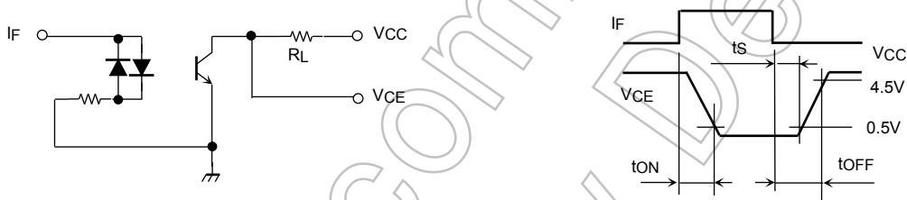
Fig. 1: Switching operating conditions
