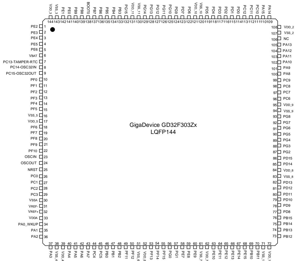
Figure 2-2. GD32F303Zx LQFP144 pinouts
